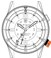
PUSH AND TURN CROWN CLOCKWISE AND SCREW DOWN
