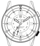
TURN CROWN ANTI- CLOCKWISE TO ADJUST GMT HAND
