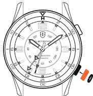
PUSH AND TURN CROWN CLOCKWISE AND SCREW DOWN
