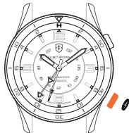
TURN CROWN ANTI- CLOCKWISE TO ADJUST GMT HAND
