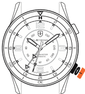
UNSCREW CROWN TO MANUAL WINDING POSITION
